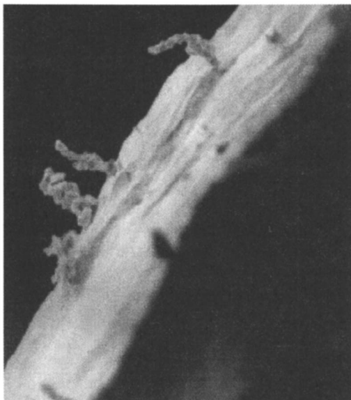
Figure 4. Ta 2 C crystals on tantalum ( T = 3200 K, P \sim 10^{-2} Pa, t = 300 s).
